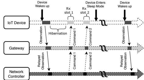
Fig. 1: Message sequence of an IoT device using LoRaWAN radio operating in class A.
