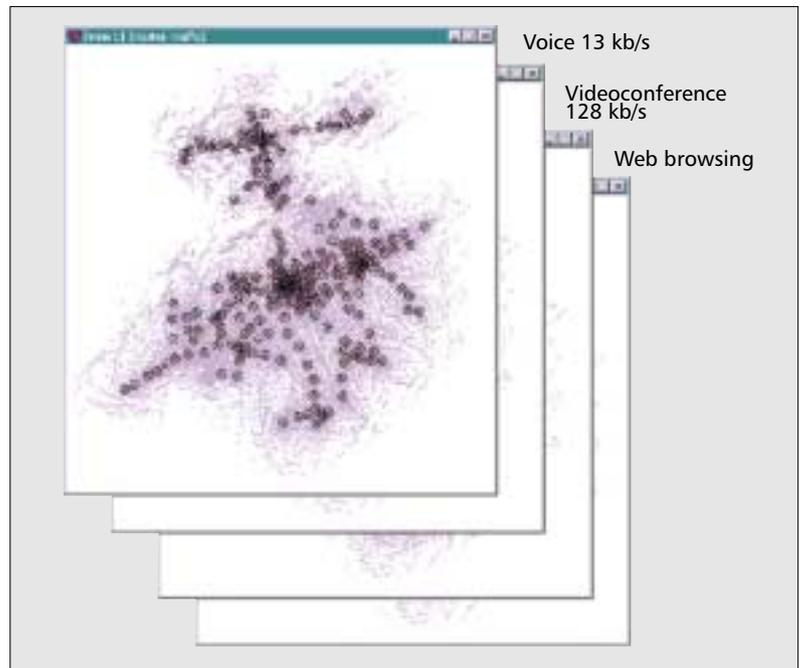
Figure 7. An example of one demand scenario for a specific time of day, with multiple traffic (user) grids (one grid for each user profile).
