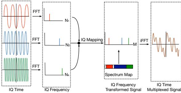
Fig. 2. Multiplexing process performed by HyDRA.
