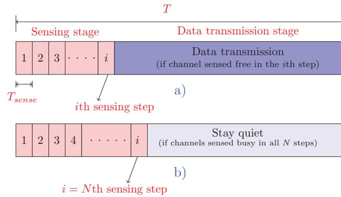
Fig. 2. Time slot structure with sensing and data transmission stages. a) If a CR finds a channel free in its  $i$ th sensing step, it transmits in that channel until the end of the slot. b) If in all sensing steps channels are sensed to be busy then the CR stays silent for the entire duration of that time slot.
