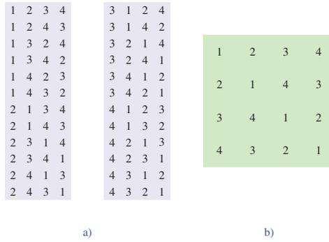
Fig. 4. Examples of sensing orders for  $N = 4$  potentially available channels. In a), the space of all permutations of  $N = 4$  channels is illustrated, while in b), a subset of that space (a Latin Square) is illustrated. A sensing order is a row of a Latin Square or a row of a permutation space of  $N$  channel indices.
