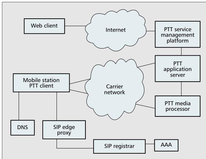
Figure 3. HP/Tobagi PacketChat architecture (adapted from [4]). DNS is the Domain Name Service module, and AAA is the authentication, authorization, and accounting module.
