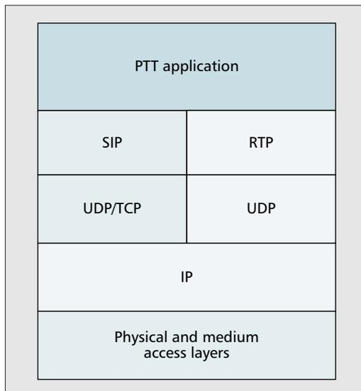
■ **Figure 2.** Protocol stack for support of PTT over VoIP.
