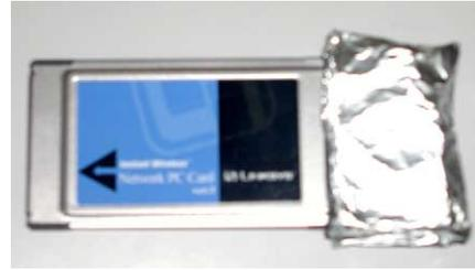
Fig. 5. Antenna portion of the wireless PC card wrapped with aluminum foil “attenuator.”
